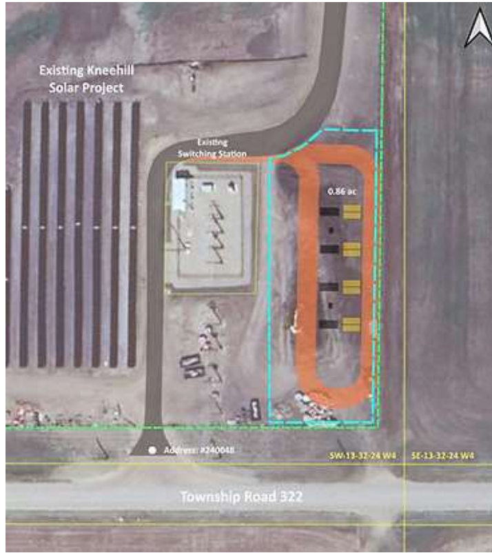
Figure 1. Location of new BESS equipment at the Kneehill Solar Project. (The blue dashed line represents the total maximum construction area, the orange areas represent new roads for emergency vehicles to go around the batteries, the yellow rectangles show the battery container locations, and the black rectangles represent the inverters and electrical equipment.)
